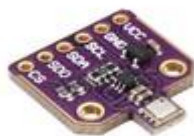
CJMCU-680 BME680 TEMPERATURE HUMIDITY AIR PRESSURE I2C
