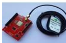
GPS SHIELD SKG13C WITH 3 METER ANTENNA
