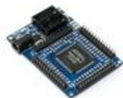
ALTER EP2C5T144 FPGA CYCLONE BOARD
