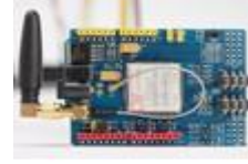
GSM SHIELD SIM900A WITH 2BDI ANTENNA
