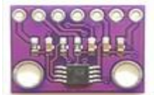
AD8221AR INSTRUMENTATION AMPLIFIER MODULE
