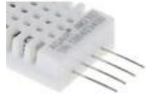
DHT22 TEMPERATURE HUMIDITY MODULE
