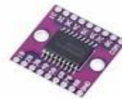
CJMCU-2803 ULN2803A DRIVER MODULE
