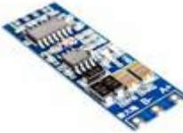
MAX485 TO TTL RS485 FUSE CONVERTER
