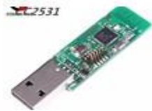
CC2531 SNIFFER USB DONGLE
