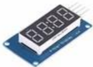
TM1637 4BIT DIGITAL LED TUBE DISPLAY
