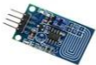
PWM CAPACITOR TOUCH DIMMER
