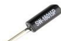
SW-18015P VIBRATION SWITCH MODULE
