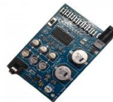
APR33A3 RECORDING VOICE PLAYBACK
