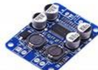
TPA3118 PBTL MONO 60W DIGITAL AMPLIFIER
