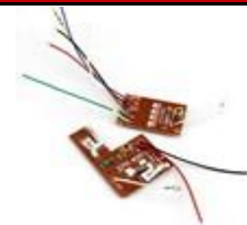
4CH REMOTE CONTROL TRANSMITTER RECEIVER CIRCUIT
