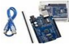
ARDUINO UNO SMD CH340 USB IC A TO B CABLE ACRYLIC CASE
