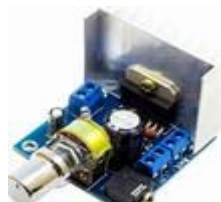
TDA7297 15W DUAL AMPLIFIER BOARD
