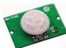
GH-718 PIR HUMAN BODY SENSOR DIGITAL
