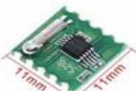
RDA5807M FM STEREO RADIO V2.0
