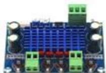
XH-M572 TPA3116D2 120W DIGITAL POWER AMPLIFIER
