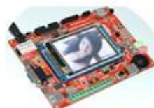
STM32F103ZET6 M3 ARM CORTEX STM32 DEVELOPMENT BOARD
