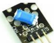
KY-020 TILT SWITCH SENSOR
