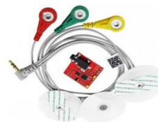
EMG MUSCLE SENSOR V3.0 DIGITAL
