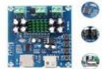
XH-M422 TPA3116D2 BLUETOOTH AMPLIFIER 50W
