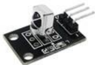
KY-022 IR RECEIVER DIGITAL TSOP
