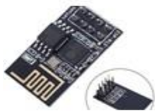
ESP-01 ESP8266 SERIAL WIFI TRANSCEIVER MODULE
