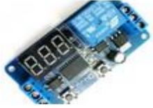
DELAY TIMER CONTROL 12V RELAY LED DISPLAY
