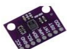
CJMCU-811 CCS811 AIR QUALITY MOINTORING INDOOR I2C DIGITAL
