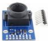
MCU-115 TCS3414CS COLOR RECOGNITION DETECTOR I2C
