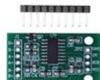
HX711 24 BIT AD LOAD CELL WEIGHING AMPLIFIER
