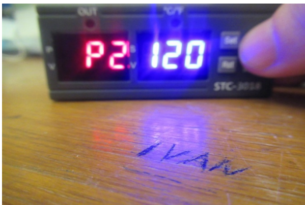
Max temperature alarm
