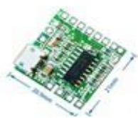
PAM8303 3W DUAL CHANNEL CLASS D MICRO USB
