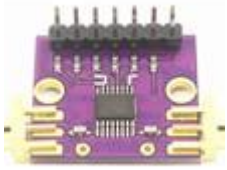
CJMCU-274 HMC274 ATTENUATOR WIDEBAND GAAS 0.7 2.7GHZ
