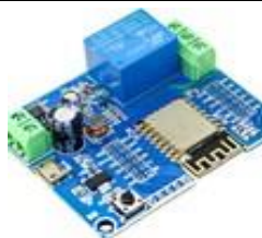
AC 220V ESP-12S 1 CHANNEL WIFI RELAY BOARD
