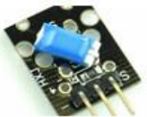
KY-020 TILT SWITCH SENSOR
