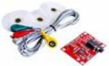
AD8232 ECG HEART RATE MONITOR ANLOG
