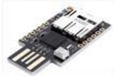
CJMCU VIRTUAL KEYBOARD USB TF STORAGE ATMEGA32U4
