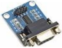
DB9 FEMALE RS232 TO TTL BREAKOUT 4 PIN
