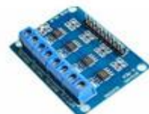
L9110S 4 CHANNEL MOTOR DRIVER
