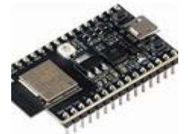
ESP32-C3-DEVKITM-1 WITH ESP32-C3-MINI-1-N4 MODULE
