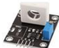
WCS1800 35A HALL OVER CURRENT PROTECTION ANALOG VOLTAGE
