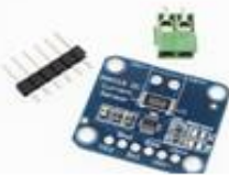
CJMUI-219 INA219 I2C NO DRIFT BI DIRECTIONAL I2C
