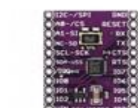
CJMCU-750 SC16IS750 UART IIC I2C SPI INTERFACE
