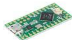
TEENSY 2 USB MICRO DEVELOPMENT BOARD
