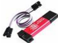
ST LINK V2 PROGRAMMER STM8 TO STM32
