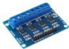
HG7881 4 CHANNEL MOTOR DRIVER
