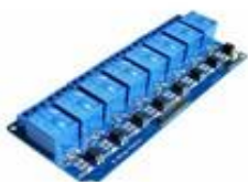
8 CHANNEL 12V OPTO COUPLER RELAY
