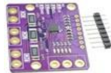
CJMCU-3221 INA3221 3 WAY BI DIRCTIONAL I2C
