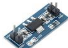
AMS1117 1.8V POWER SUPPLY MODULE DC DC
