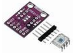
CJMCU-101 MCU101OPT101 MONOLITHIC PHOTO M6A2 I2C
