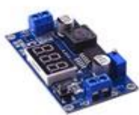
XL6009 4A BOOST LED DISPLAY VOLTMETER
