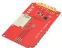
2.8 INCH TFT SPI 240X320 WITHOUT TOUCH
