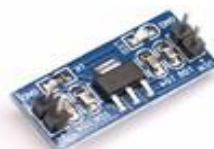
AMS1117 1.5V POWER SUPPLY MODULE DC DC
