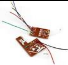
4ch Remote Control Transmitter Receiver Circuit
