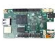
UDOO NEO EXTENDED SINGLE BOARD COMPUTER
