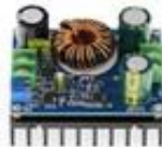
600W 10A 10-60V TO 12-80V BOOST MODULE
