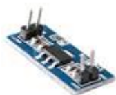
AMS1117 2.5V POWER SUPPLY MODULE DC DC
