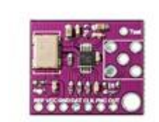
CJMCU-9833 AD9833BRMZ SINE SQUARE WAVE
