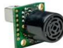
MB1200 XL-MAXSONAR-EZ0 ULTRASONIC PWM
