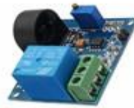
5A 12V AC DC OVER CURRENT PROTECTION
