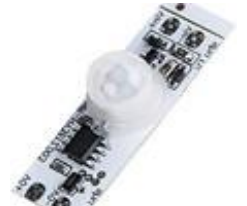
HY-3612 V1.0 PIR MOTION SENSOR 12 24V SWITCH
