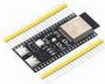
ESP32 S3 WROOM-1-N16R8 ESP32-S3-DEVKITC-1
