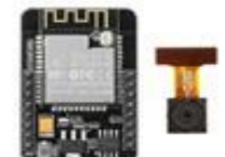
ESP-32 CAMERA OV2640 2MP FACE RECOGNITION
