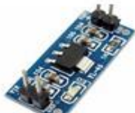
AMS1117 1.2V POWER SUPPLY MODULE DC DC
