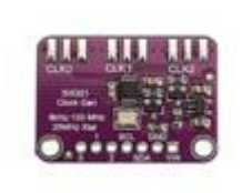
GY-5351 SI5351 SIGNAL SQUARE WAVE FREQUENCY
