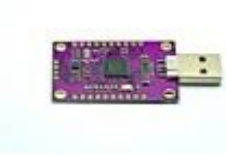
FT232H USB TO JTAG UART FIFO SPI I2C
