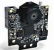
PIXY 2.1 SMART VISION SENSOR OBJECT TRACKING CAMERA
