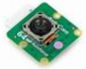
ARDUCAM 64MP AUTOFOCUS CAMERA MODULE
