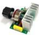
3000W THYRISTOR SCR DIMMER FOR SPEED LIGHT
