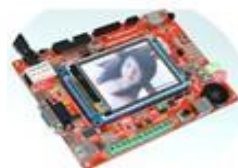
STM32F103ZET6 M3 ARM CORTEX STM32 DEVELOPMENT BOARD
