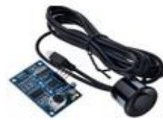
JSN SR04T WATERPROOF ULTRASONIC WITH PROBE PWM
