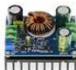
600W 10A 10-60V TO 12-80V BOOST MODULE
