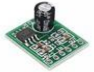
XH-M125 XPT8871 6W MONO AMPLIFIER BOARD
