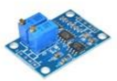
AD620 MICROVOLT MILIVOLT HIGH PRECISION AMPLIFIER
