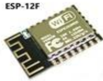
ESP-12F ESP8266 WIFI WIRELESS TRANSCIEVER
