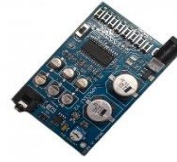
APR33A3 RECORDING VOICE PLAYBACK
