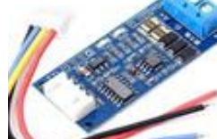
RS485 TTL FOR SOIL NPK SENSOR
