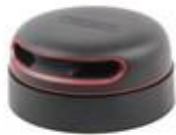
RPLIDAR A2M6 360 DEGREE LASER RANGE FINDR 18M
