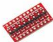
BI DIRECTIONAL LOGIC LEVEL CONVERTER 8 CHANNEL
