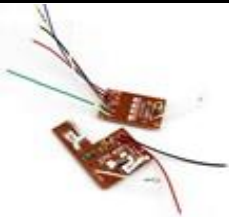
4ch Remote Control Transmitter Receiver Circuit
