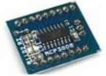
MCP3008 PI ADC BREAKOUT BOARD
