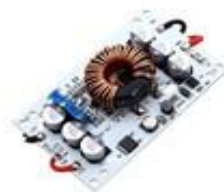
600W ALUMINUM BOOST CONT VOLT CONT CURRENT
