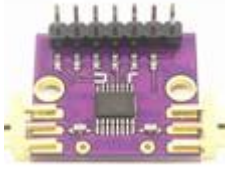
CJMCU-274 HMC274 ATTENUATOR WIDEBAND GAAS 0.7 2.7GHZ
