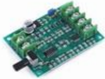
BLDC MOTOR DRIVER 7 12V HARD DRIVE 3/4 WIRE
