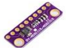
GY-ADS1015 ADS1015 12 BIT 4 CHANNEL ADC
