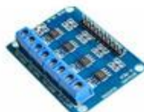
L9110S 4 CHANNEL MOTOR DRIVER
