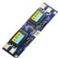
CCFL INVERTER BOARD 10- 28V HIGH VOLTAGE HIGH PRESSURE FOR 4 BULBS
