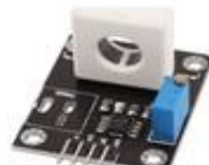
WCS1800 35A HALL OVER CURRENT PROTECTION ANALOG VOLTAGE
