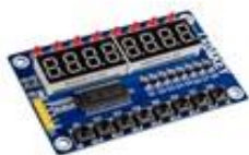
TM1638 8DIGIT DIGITAL LED DISPLAY WITH BUTTON
