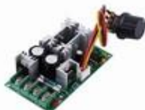
40A 12-48V PWM DC MOTOR SPEED REGULATOR
