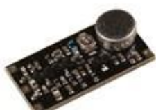
FM TRANSMITTER 85 115MHZ 100M 800M
