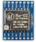
AI THINKER SX1278 LORA RA-02 433MHZ WITH BASEBOARD
