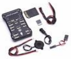
PIXHAWK 2.4.8 FLIGHT CONTROLLER 32BIT AUTOPILOT
