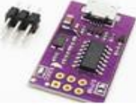
HW-534 ATTINY44 5V MICRO USB DEVELOPMENT BOARD
