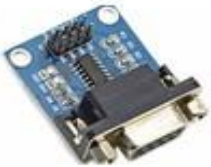
DB9 FEMALE RS232 TO TTL BREAKOUT 4 PIN
