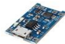
TP4056 1A 5V LI-ION BATTERY PROTECTION 18650 MICRO USB
