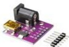
CJMCU-MINI USB 5-12V TO 3.3V SOCKET USB DC AMS1117
