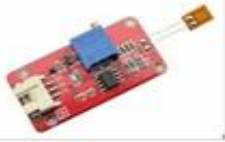
STRAIN GAUGE Y3 WEIGHING AMPLIFIER MODULE
