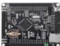
STM32F407VET6 M4 ARM CORTEX STM32 DEVELOPMENT BOARD
