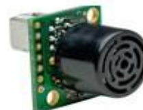
MB1200 XL-MAXSONAR-EZ0 ULTRASONIC PWM
