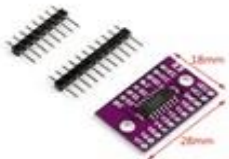
CJMCU-4051 74HC4051 8 CHANNEL ANALOG MULTIPLEXER
