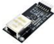
LAN8720 ETHERNET TRANSCIVER RMII INTERFACE
