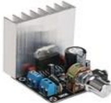
TDA7377 35W DUAL AMPLIFIER BOARD
