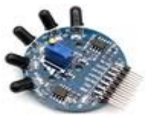
5 CHANNEL FLAME DETECTION MODULE DIGITAL
