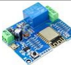
AC 220V ESP-12S 1 CHANNEL WIFI RELAY BOARD
