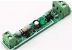
1 CHANNEL 220V AC OPTOCOUPLER ISOLATION
