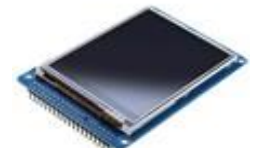
3.2 INCH TFT TOUCH DISPLAY RASPBERRY PI
