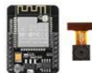
AI THINKER ESP32 CAMERA OV2640-R-4586
