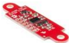
VL6180 LASER TOF FLIGHT TIME RANGING
