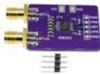
AD8302 RF LOGARITHMIC DETECTOR
