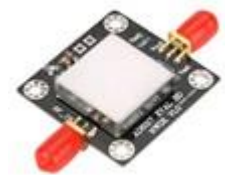
AD831 60DB 1M 10GHZ RF LOGARITHMIC DETECTOR
