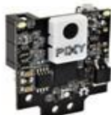
PIXY 2 SMART CAMERA OBJECT TRACKING
