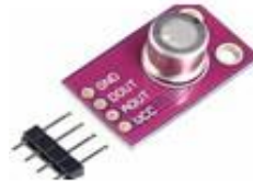
MS-1100 FORMALDEHYDE BENZENE GAS SENSOR ADC
