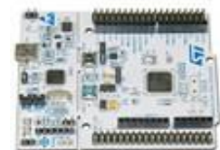
NUCLEO-F401RE STM32F401RE ARM CORTEX M4 NUCLEO 64 -PIT
