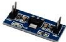
AMS1117 3.3V POWER SUPPLY MODULE DC DC
