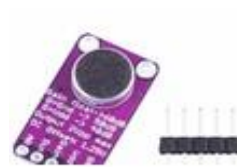
MAX9814 MICROPHONE AMPLIFIER AGC AUTO GAIN
