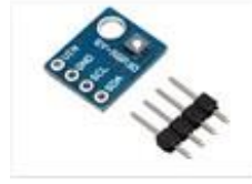
GY-SGP30 AIR QUALITY TVOC EC02 FORMALDEHYDE SENSOR
