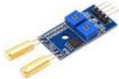
2 CHANNEL TILT SENSOR
