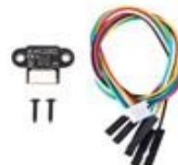
TOF10120 LASER TOF FLIGHT TIME RANGING 10 180CM
