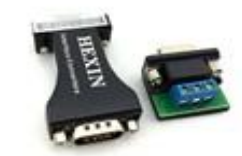
HEXIN RS232 TO RS485 INTERFACE ADAPTER
