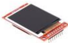
1.8 INCH TFT LCD COLOR 128X160 4 PIN
