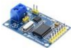
TJA1050 MCP2515 CAN PROTOCOL SPI MODULE
