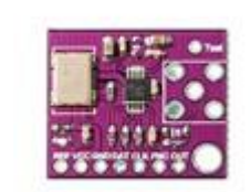
CJMCU-9833 AD9833BRMZ SINE SQUARE WAVE
