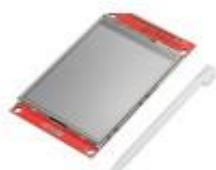
2.8 INCH TFT SPI 240X320 WITH TOUCH
