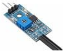
SW-18015P VIBRATION SWITCH SENSOR
