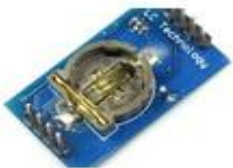
DS1307 RTC DS18B20 TEMPERATURE I2C
