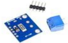
GY-169 INA169 ANALOG CURRENT ANALOG VOLTAGE
