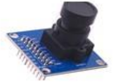
OV7670 VGA CMOS CAMERA 640X480
