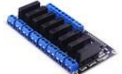
8 CHANNEL 5V SSR RELAY SOLID STATE RELAY
