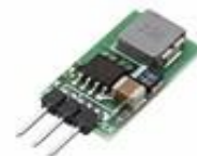
1A 5V VOLTAGE STABILIZED DC 5.5-32V
