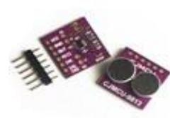
CJMCU-9813 MAX9813H MICROPHONE AMPLIFIER
