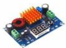
XH-M411 5A 3-35V TO 5-45V LED DISPLAY
