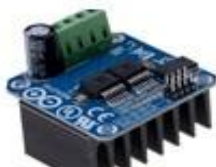
BTS7960 43A H-BRIDGE MOTOR DRIVER
