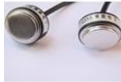
ULTRASONIC FLOW METER SENSOR PWM
