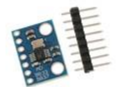
GY-9833 AD9833 PROGRAMMABLE DDS SIGNAL GENERATOR
