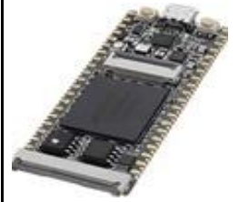
SIPEED TANG PRIMER FPGA DEVELOPMENT BOARD
