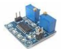
TL494 PWM TO FREQUENCY 500-100KHZ 250MA
