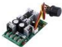
20A 12 48V PWM DC MOTOR SPEED REGULATOR
